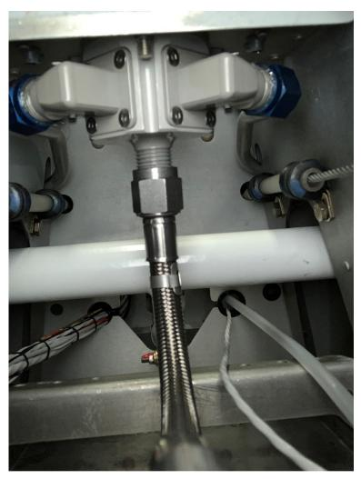
Standard Valve (Andair Type 2) – Wing Root filter setup – For this setup you will receive a new hose that goes from the Valve to the Pump and from the pump to the firewall
