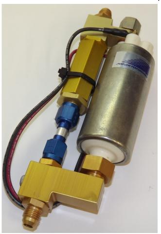
up and running, please note that the side of the filter with the DOUBLE HEX is the output side of the filter and and needs to go into the input side of the fuel pump. We recommend drawing an arrow on the filter to show flow direction so there is no confusion during servicing.
