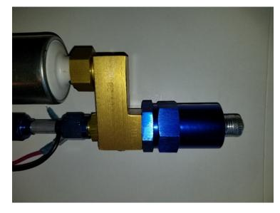
VERY IMPORTANT: When removing the gold AN fitting, there is a gasket that needs to be transferred to the fuel filter prior to screwing it into the pump assembly. Failure to do this will result in leakage.
